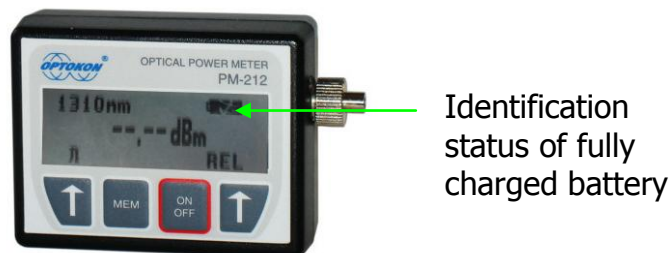
Figure 2: Status of fully charged battery
